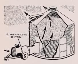
designed and big enough for the work. These machines should also have automatic controls to stop fuel flow if the burner flames go out.
